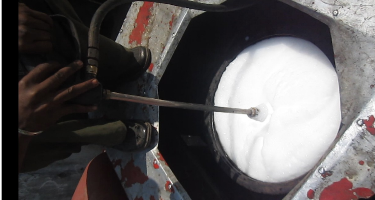
Figure 3: Thick foaming from Freshin 10 X diluted solution after aeration with the pump
